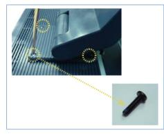
Remove 4 screws and then remove hinge.
